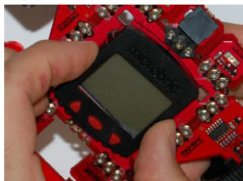
Clean the contact on the motherboard, preferably with a lint free cloth and some audio/video head cleaning solution. An alternative would be a cotton bud and methylated spirits, but ensure there are no fibres left on the board from the cotton bud.
