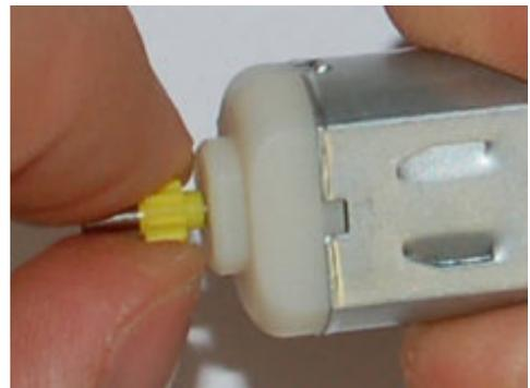
Use a 5c coin or similar to lever the pinion gear away from the motor about half a millimetre, so it can spin freely.
